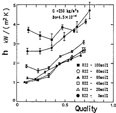
FIG. 3. Boiling heat transfer coefficient as a function of steam quality at different compositions, for R 22/R 114 mixtures (Hihara and Saito [7]).
