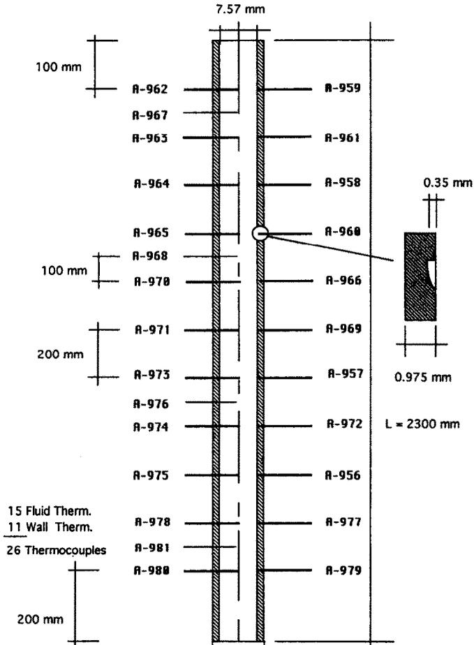
FIG. 5. Schematic of the THOM test section (ENEA).
