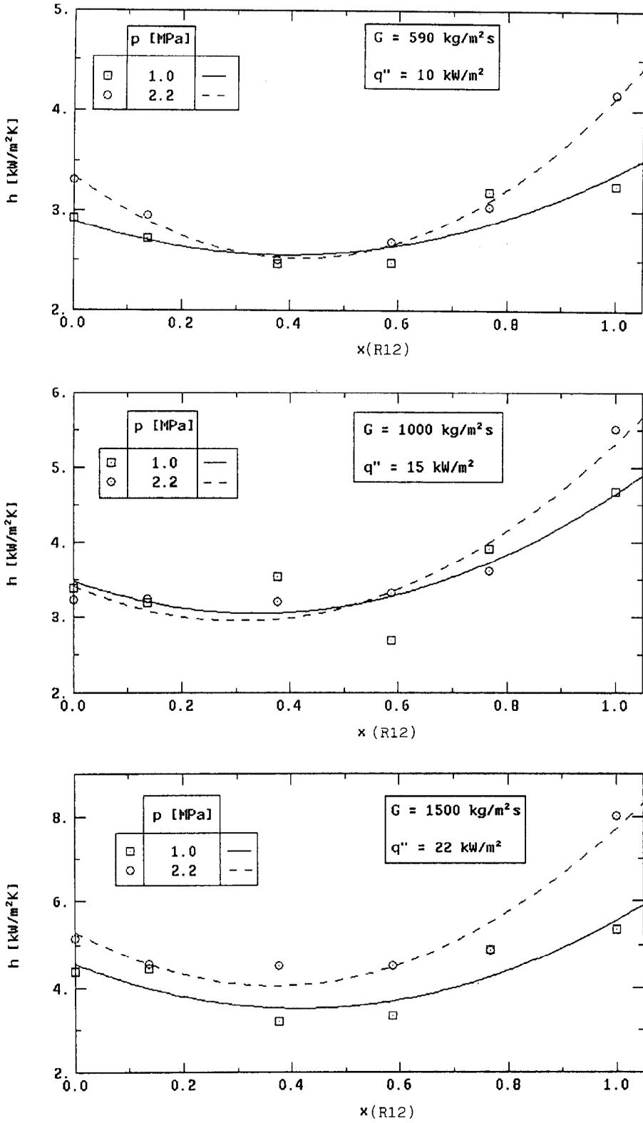
FIG. 7. Heat transfer coefficient as a function of composition at various mass fluxes and pressures, for R 12/R 114 mixtures (ENEA).
