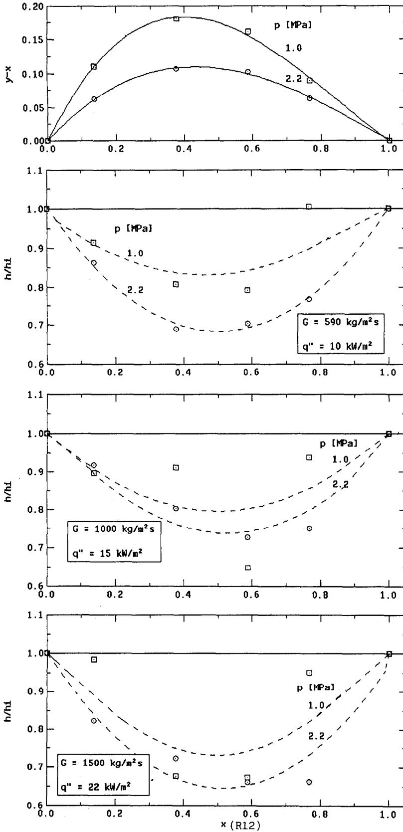
FIG. 6. Vapour/liquid mole fraction difference as a function of composition (top graph) and relative decrease of the heat transfer coefficient as a function of composition at various mass fluxes and pressures, for R 12/R 114 mixtures (ENEA).
