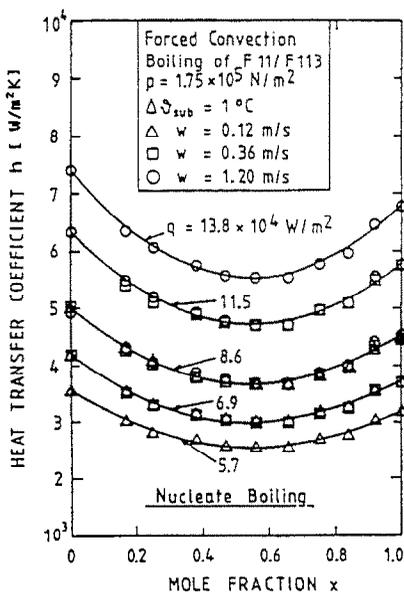
FIG. 1. Boiling heat transfer coefficient as a function of composition at different liquid velocity and heat flux, for R 11/R 113 mixtures (Fink *et al.* [3]).
