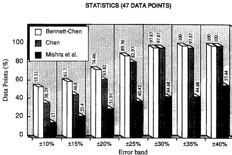
FIG. 9. Comparison of different heat transfer correlation performances using different mass fluxes, pressures and composition of R 12/R 114 mixtures, as detailed in the test matrix (ENEA).
