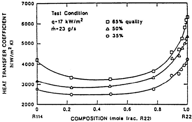
FIG. 2. Boiling heat transfer coefficient as a function of composition at different steam quality, for R 22/R 114 mixtures (Jung *et al.* [5]).
